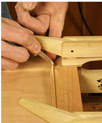
The quarter-round molding is shaped on the router, then mitered to fit the door. Becksvoort simply glues the molding to the rails and the stiles.
